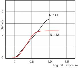
Sensitometric parameters according to ISO standard:
